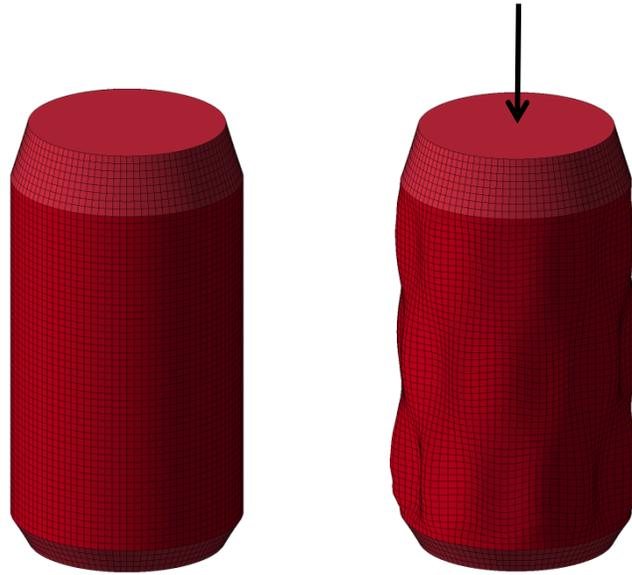
Figure 3735-1 Linear axial buckling of an aluminium beverage can.
